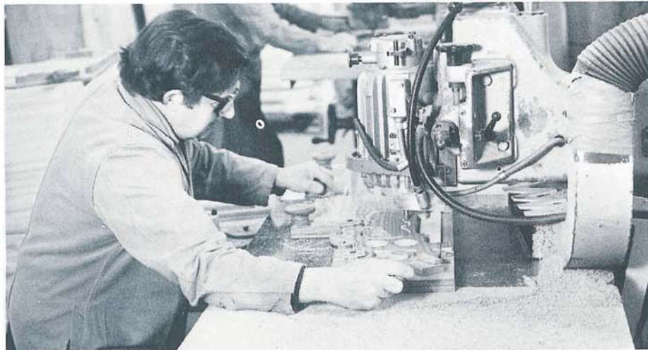
6 Routing out the inner profiles of a facia panel
