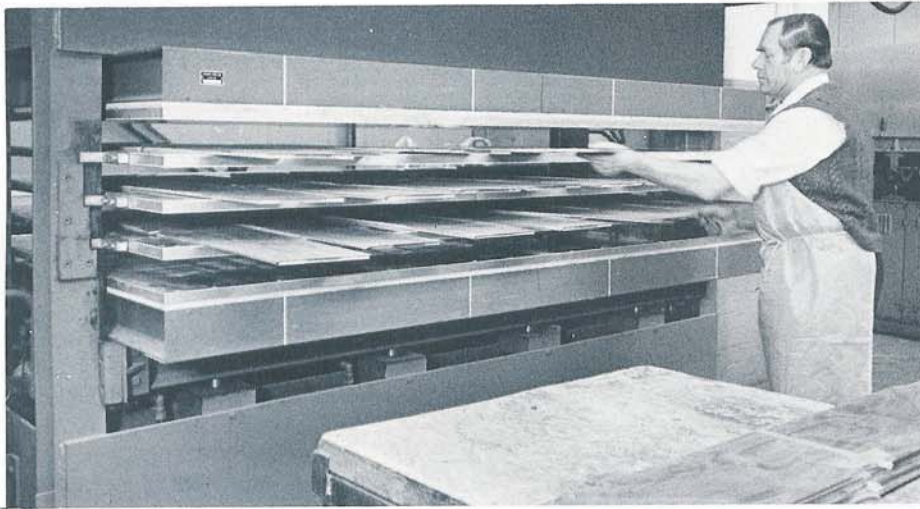
4 Placing the panels in the multi-daylight press
