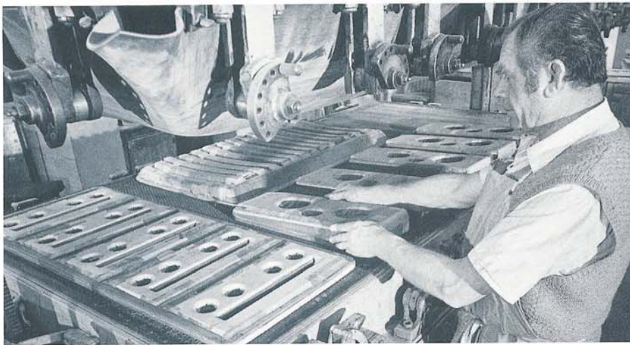
5 Veneered door trim in the vacuum press
