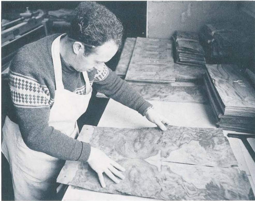
1 Mirror matching burl walnut veneer before laminating with Aerolite
