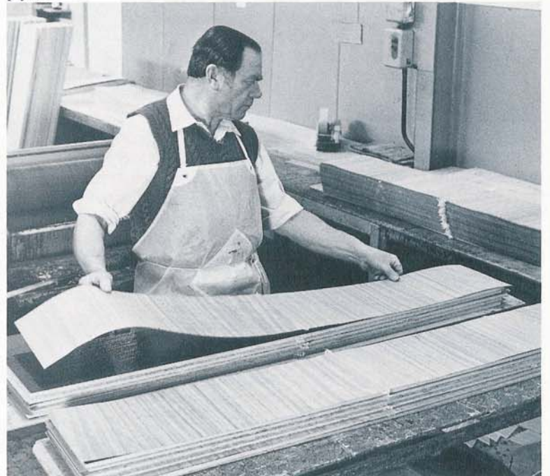
3 Laying veneer onto the Aerolite coated plywood
