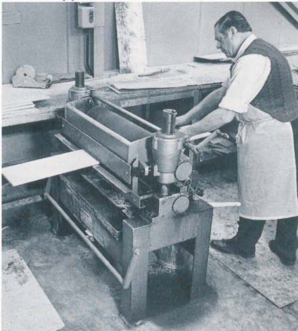
2 Aerolite adhesive being applied by roller coater to the plywood base
